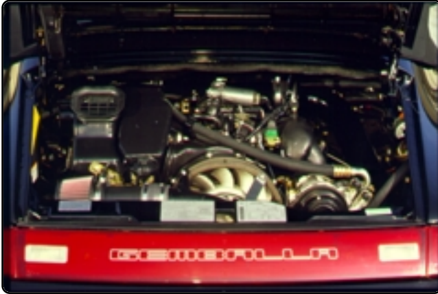
BITURBO 450 / 500 HP Water / air intercooler Basic car Carrera
