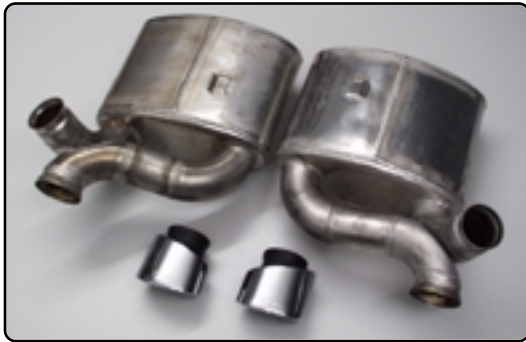
SPORT-End muffler for TURBO with 70 mm-pipes
