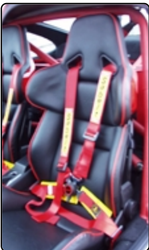
RACING-Seat with side protection, 4-point-belt (roll bar leather coverd)
