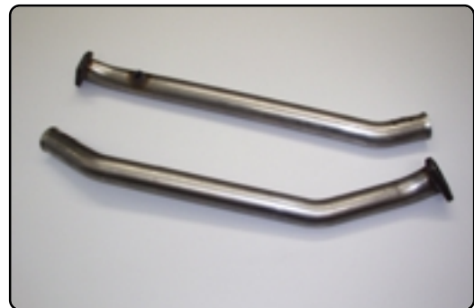
Catalysts replacement pipes for BITURBO „More power, better sound . . .“ *Export without TÜV
