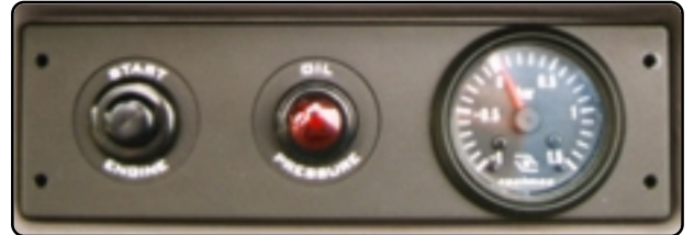
Motor-Start console with start-button, oil and turbo boost gauge
