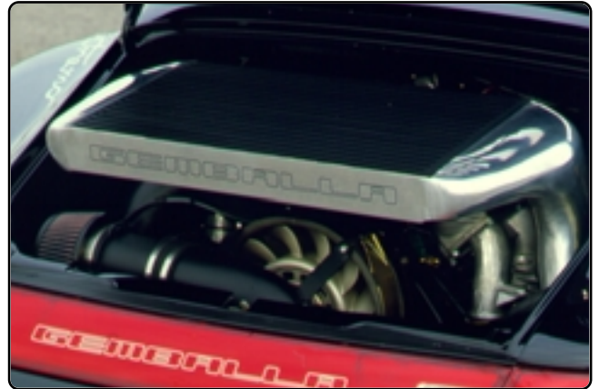
BITURBO 450 / 500 / 550 / 600 HP Air / air intercooler Basic car Carrera
