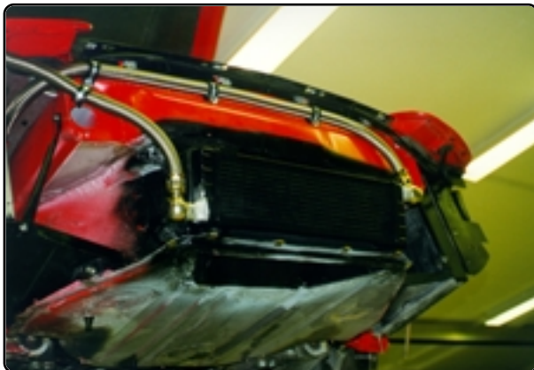
Additional oil cooler RACING (with front airintake) for highest regards
