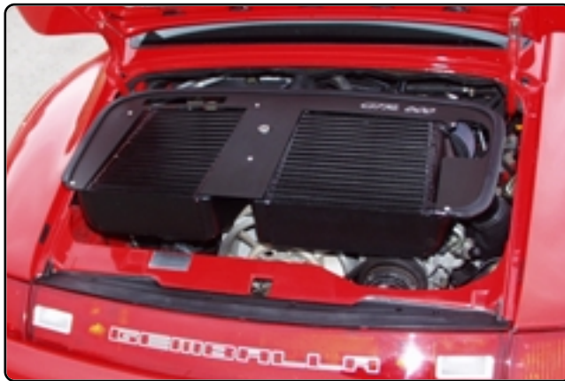
BITURBO 490 / 520 / 570 / 600 HP Air / air intercooler Basic car TURBO
